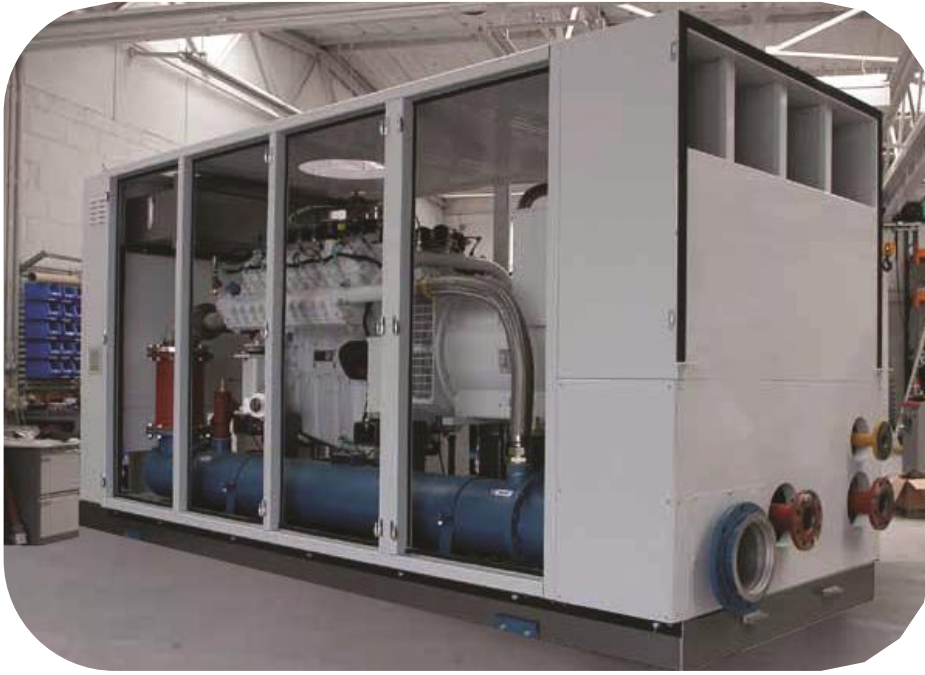
185kWe ENER-G CHP unit
