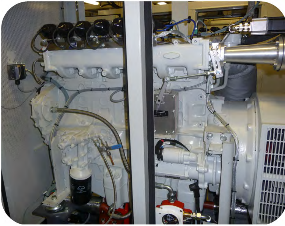
The six cylinder MAN engine with 62kWe capacity
