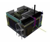
Within the energy centre, and at the request of Bausch + Lomb, a dedicated viewing platform was installed allowing site visitors to see the running engine without entering the engine room to learn more about the benefits of CHP. On-site, the CHP plant is generating electricity at 10.5kV and interfaces directly into the sites MV ring providing power to its office buildings, research and development facilities, manufacturing process and warehouse units.
